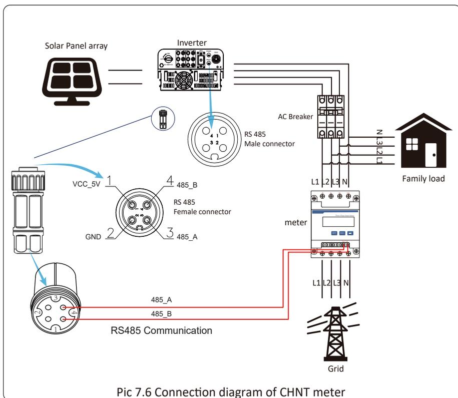
Pic 7.6 Connection diagram of CHNT meter
