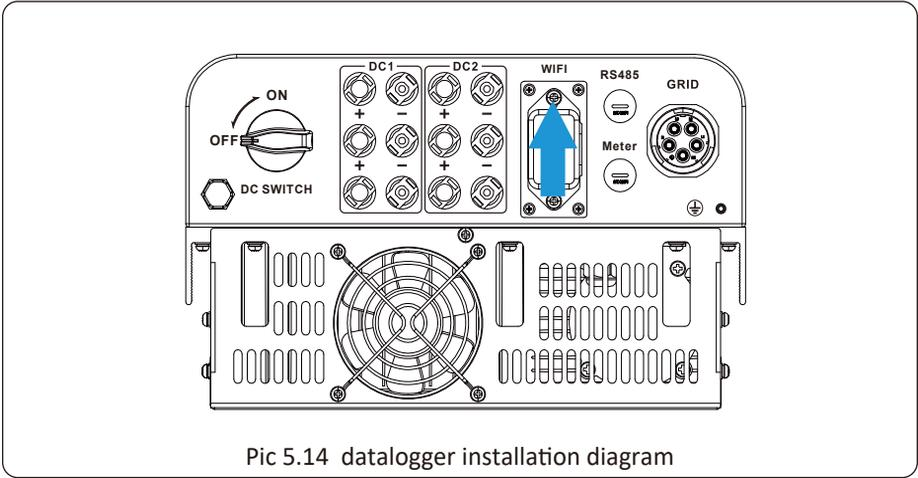
Pic 5.14 datalogger installation diagram
