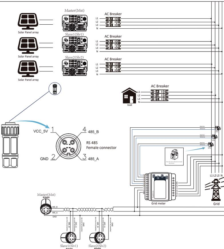
Pic 7.11 Connection diagram(Three-phase electricity )
