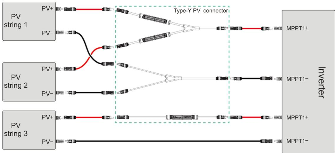
Figure3-40 Wiring diagram (connected from PV string)
