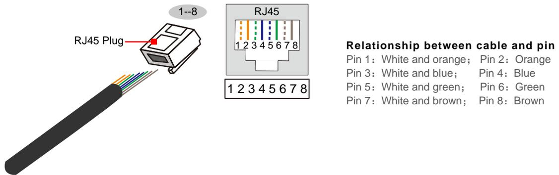
Figure3-45 Diagram of crimping of Ethernet communication wire
