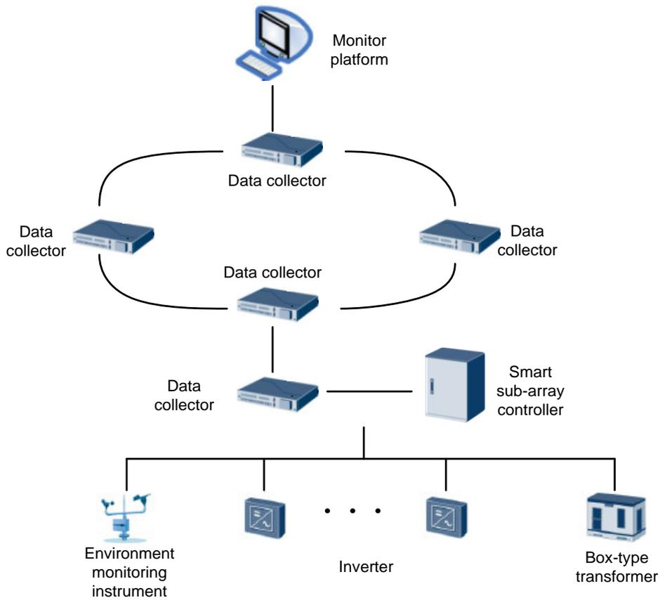
Figure2-16 Network application scheme of smart sub-array controller
