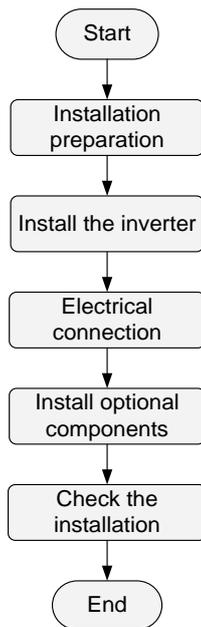
Figure3-1 Installation process
