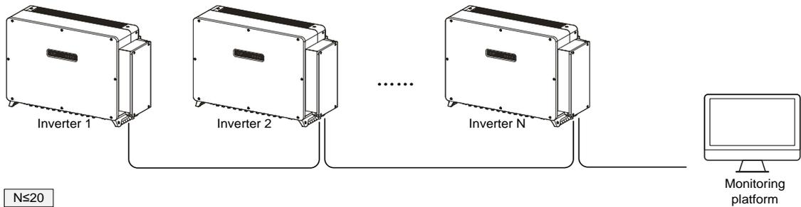
Figure2-12 RS485 communication (multiple inverters)
