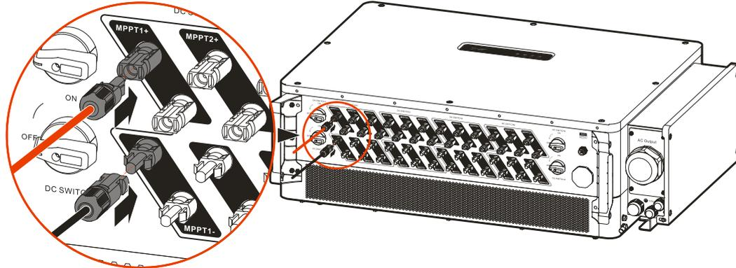
Figure3-43 Connect PV connectors
