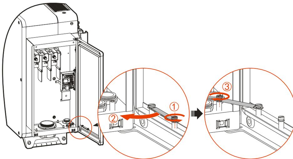
Figure3-31 Operation diagram of limiting lever
