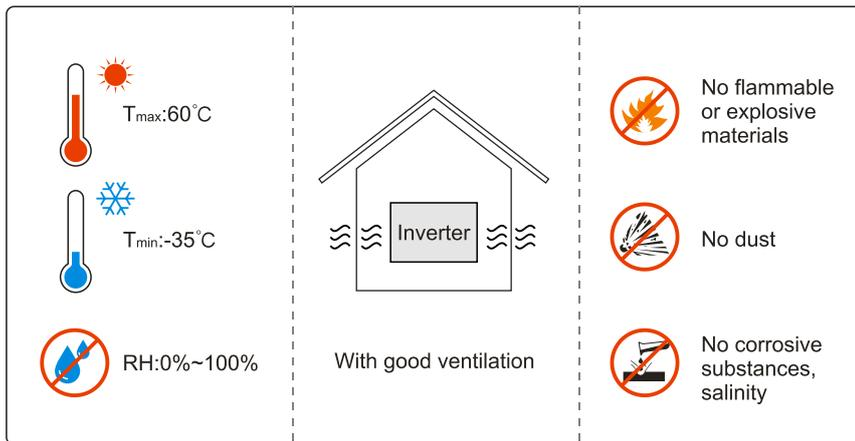
Figure3-2 Installation environment requirements
