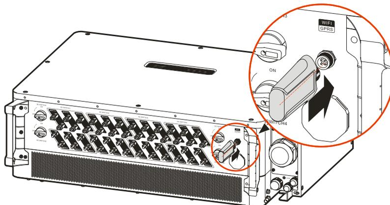
Figure3-44 WIFI/GPRS communication connection
