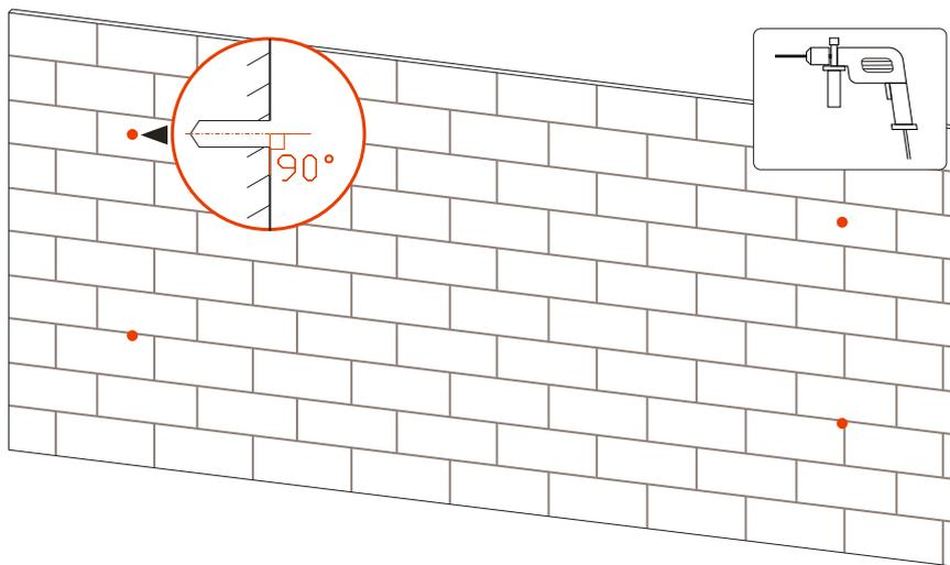
Figure3-21 Drilling holes
